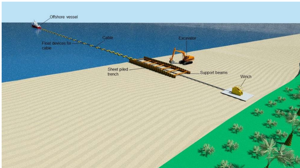
Figure 2-7: Indicative illustration of an open cut trench installation (not to scale).
